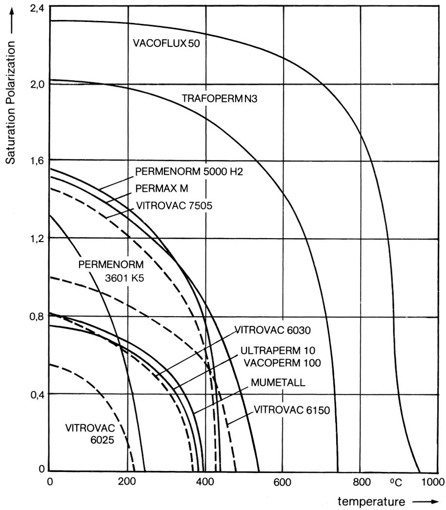
Fig. 10: Polarization Temperature Curves of Various Soft Magnetic Alloys.
