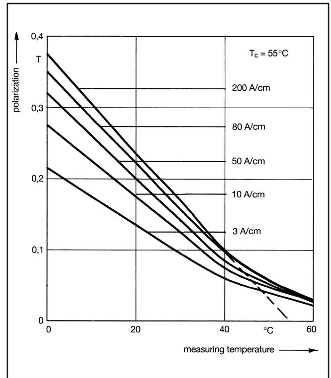
Fig. 13: Polarization Temperature Curves of THERMOFLUX 55/100 G as a Function of Field Strength ( $f = 50 \text{ Hz}$ )
