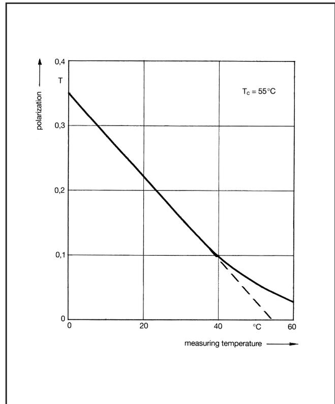
Fig. 3: Polarization Temperature Curve of THERMOFLUX 55/100-G.
