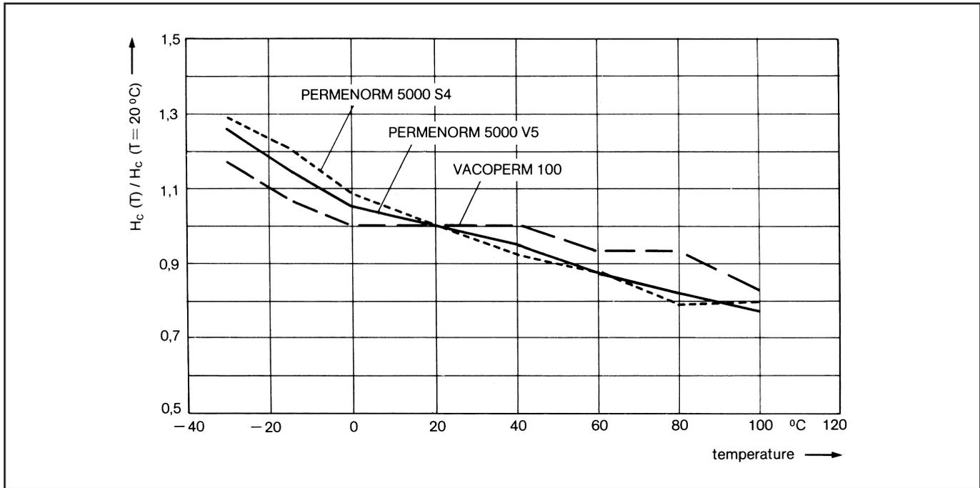
Fig. 11: Relative Temperature Dependency of Coercivity  $H_c$  (Standardized to  $20^{\circ}\text{C}$ ) of PERMENORM 5000 V5, PERMENORM 5000 S4 and VACOPERM 100.
