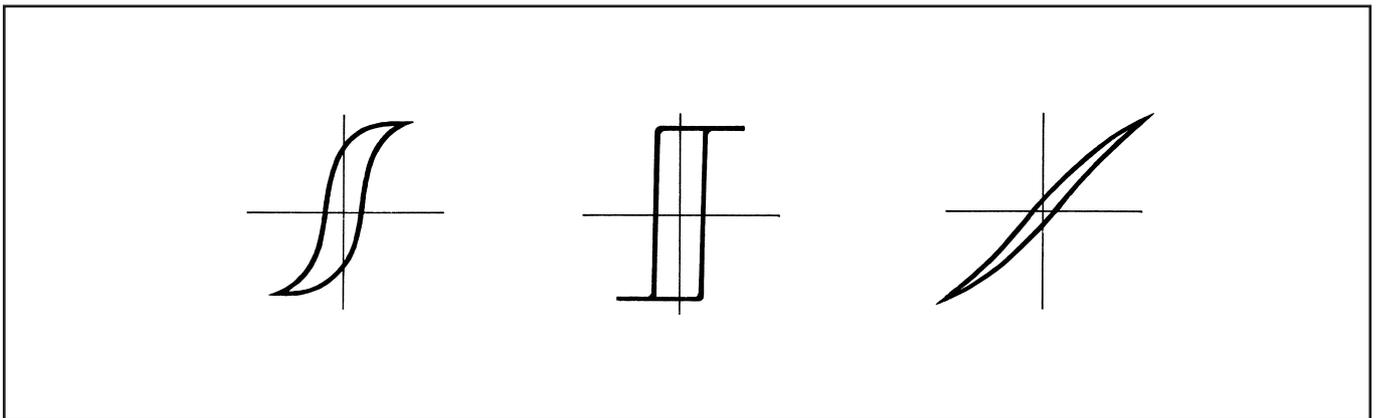
Fig. 1: Examples of Possible Hysteresis Loop Shapes in NiFe Alloys
