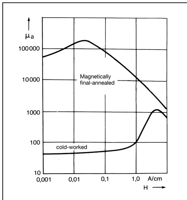
Fig. 6: The Effect of Final Heat Treatment on MUMETALL
