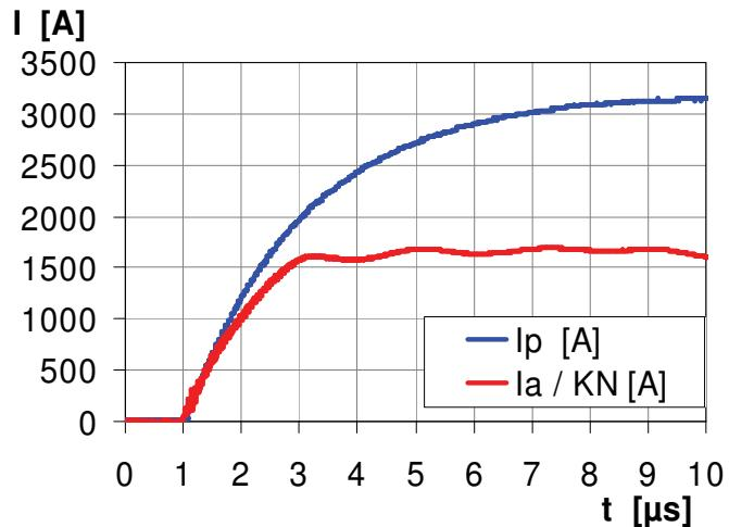
Fast increasing currents (higher than the specified  $I_{p,\max}$ ), e.g. in case of a short circuit, can be transmitted because the currents are transformed directly and be limited by diodes only.
