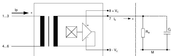
**Possibilities of wiring for  $V_C = \pm 15V$**  (@  $T_A = 70^\circ C$ ,  $R_M = 15 \Omega$ )
